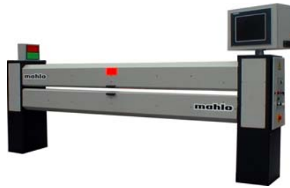
Fig.15 Compact traverse assembly
