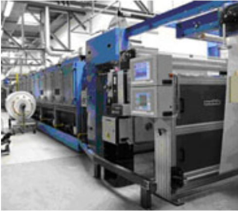
The Webscan WIS-12 can be combined with the Colorscan CIS-12. Shown here is Switzerland's Schoeller Textil AG, where the combo is used to scan for web and color faults down-stream of a washing machine with dryer.
