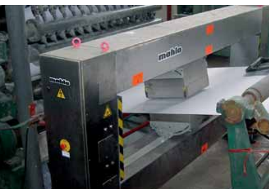
Utilizing the Ashpro FMA in paper manufacturing with large proportions of sugarcane fibres.
