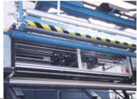
An modular straightener MFRC at the delivery side of a stenter
