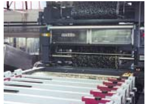
An modular straightener MFRC with a traverse assembly supported by stands (at the printing machine)
