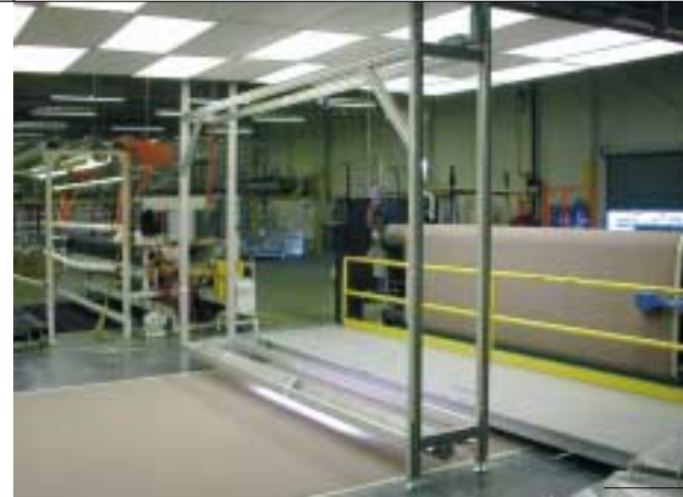
Carpet inspection PRS
