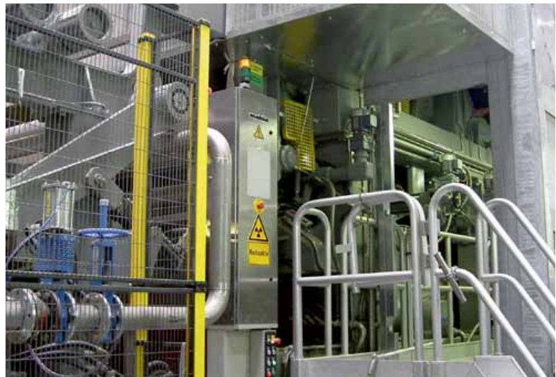
Mahlo® PaperPro II frame integrated in Tissue Line
