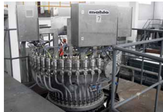
Mahlo® Qualicross: CD basis weight Profile Actuator for dilution water headbox systems.
