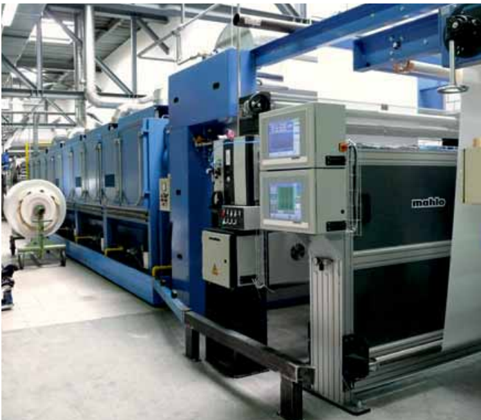
Webscan WIS-12 and colour monitor Colorscan CIS-12 at the back-end of a washing range + dryer (by kind permission of Schoeller Textiles AG, Switzerland).
