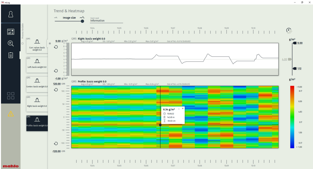
Digital Twin: Thanks to the heat map, the quality profile of the goods can be analyzed to the centimeter.
