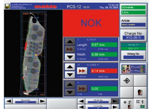
The scanner has registered a fault on the patch
