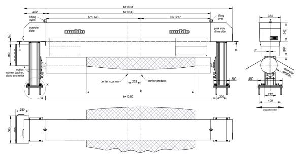
Scanning frame Uniscan M / Sensor Gravimat FMX 91-013784-02
