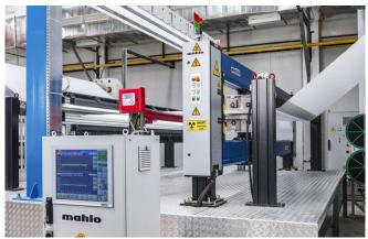
The traversing measuring frame of the Qualiscan QMS allows generating precise lateral and longitudinal profiles of parameters such as basis weight, thickness or moisture. They are presented clearly arranged in the operating software of the Mahlo system on a touchscreen (in the foreground).
