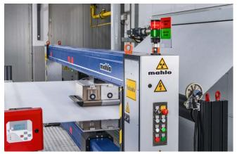
A Qualiscan QMS with a Webpro M measuring frame measures basis weight with beta sensor and moisture with an infrared sensor.
