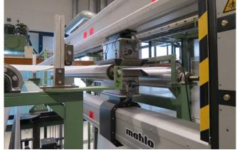
The beta sensor measures basis weight via isotope rays. Complete insensitivity to web flutter across the entire measuring gap through DFI technology (Dynamic Flutter Independent). Even smallest beta ray sources thereby achieve their maximum measuring performance.
