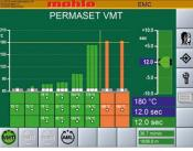
When wet product enters the dryer, it first heats up to the cooling limit temperature. At a certain temperature threshold – called the fixing temperature – the temperature necessary for processing, fixing or condensing is reached.
