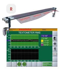
In the area of residual moisture, the conductivity of the textile substrates' water content depends most strongly on the electrically measurable properties. The residual moisture can be determined directly by measuring the electrical conductivity.
