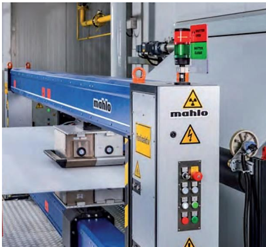
Nonwoven Manufacturer controls Basis Weight and Moisture on Spunlace Lines with Qualiscan QMS from Mahlo
