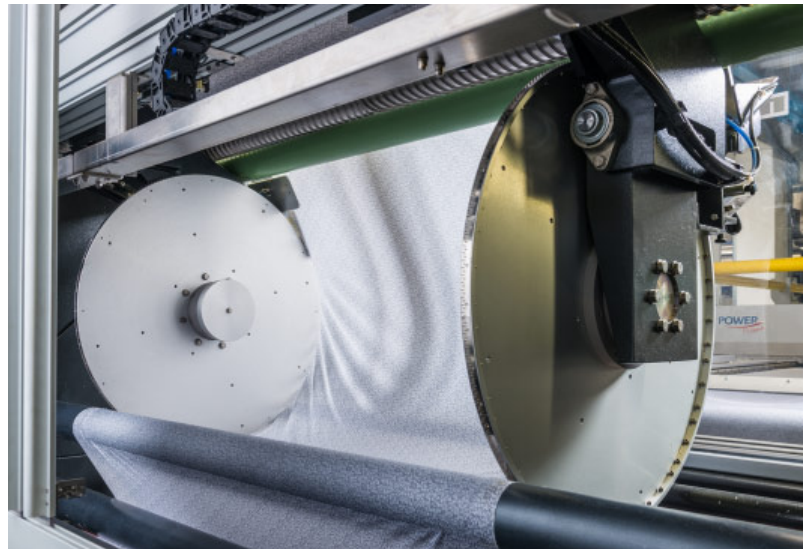
The patented adjustable unclipping roller stands out among the pin wheels. It minimises residual bow and edge distortions when unclipping the web.
