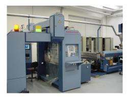
For the entire gamut of web based extruded products, whether they be cast film or extrusion coated papers or films, Mahlo makes a QCS - quality control system tailored for your specific measurement and control needs. Fixed, single-sided and dual-sided scanning platforms are available with multiple synchronized scanners are available.
