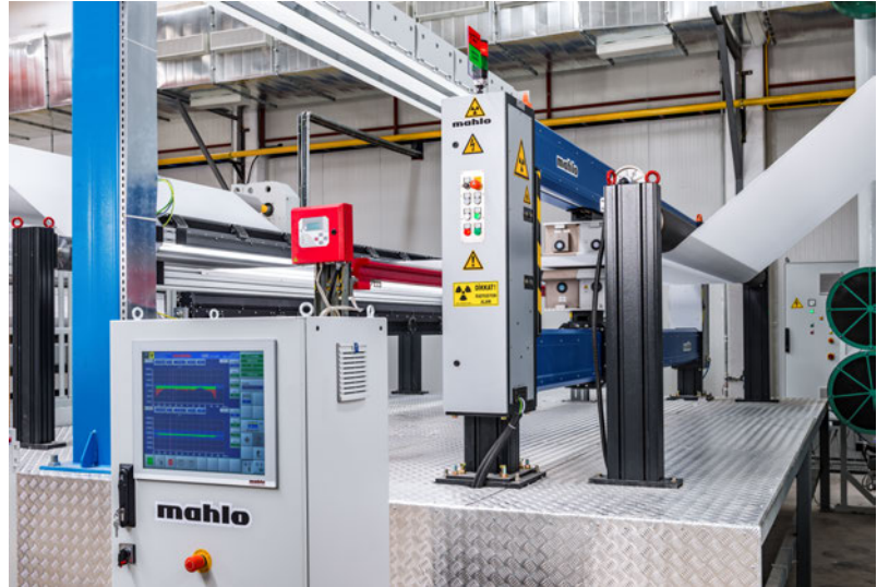
Control of basis weight and moisture on a Spunlace-Nonwoven system (courtesy of Selcuk Iplik Sanayi ve Ticaret A.S.)
