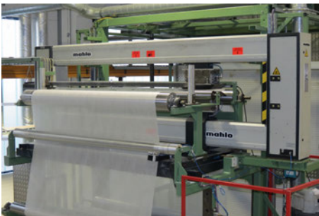
Basis weight control with the production of screen reinforcements from glass fibres and nonwovens (courtesy of Kirson Industrial Reinforcements GmbH)
