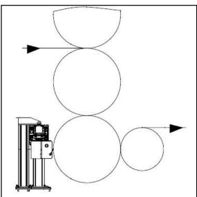
Example of an installation schemtic of a MAHLO FMX on a 3-roll calender
