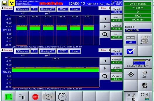
The standard Mahlo Automatic Lane Detection Tool displays only the basis weight, thickness, width and statistical information of each lane without showing the substrate. This allows for a clear and immediate understanding of the coating quality in Real Time!
