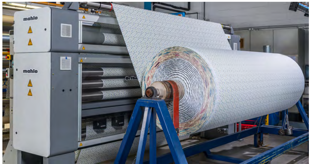
Fig. 1: New Generation Orthopac RVMC-15 with drive station MMA (photo courtesy of Stamperia Olonia)
