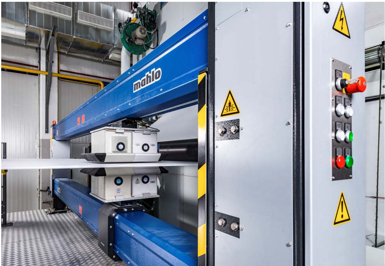
Fig. 2: Measuring of basis weight and moisture with Infracot IMF and Beta sensor on spunlace nonwoven
