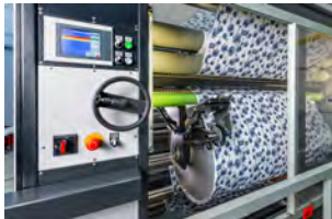
Fig. 1: Orthomax RFMB-15: Fusion of Pin-wheel and Roller Straightener
