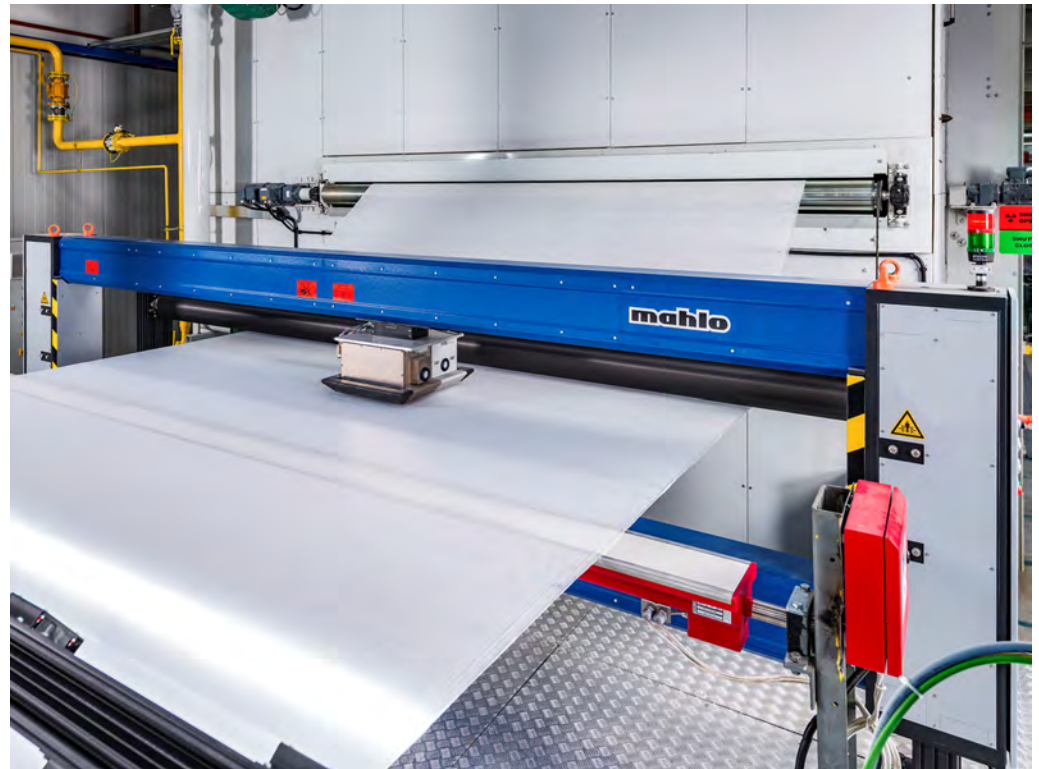
Fig. 3: Measuring Spunlace Nonwovens with Infrared Sensor Infracot IMF
