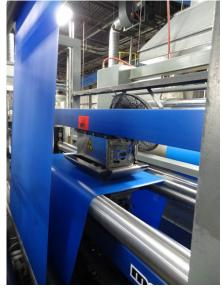
micrometer to evaluate competitor's products, the Mahlo system can print out documentation that shows the gauge consistency of Impact's plastic sheet when compared to other plastic sheet manufacturers.
