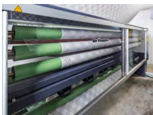
Fig. 3: Straightening with the Mahlo Orthopac RVMC
