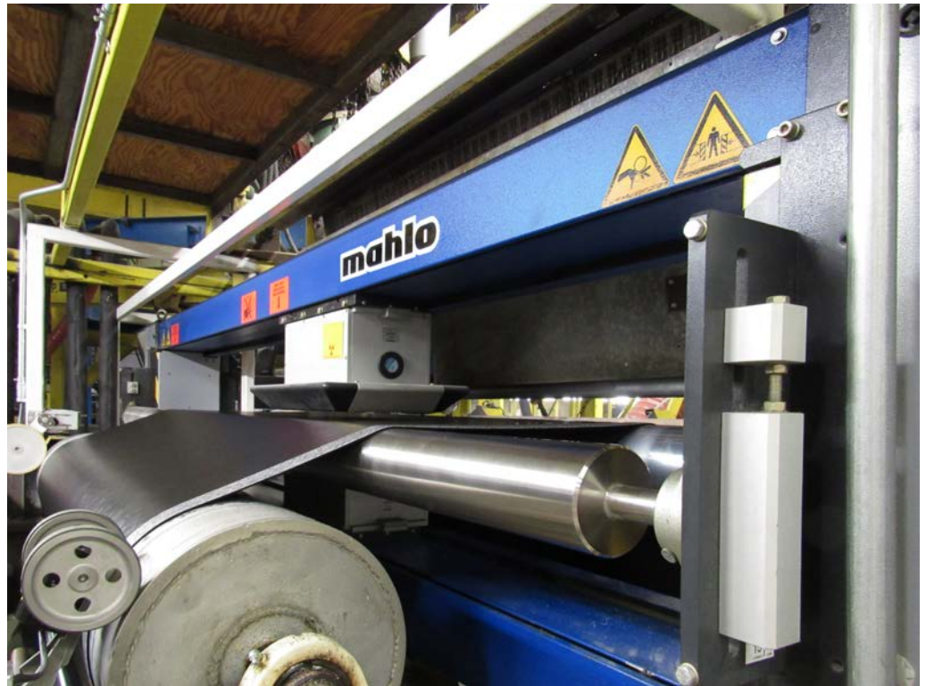
Fig. 7: Web gauging with DFI Sensor
