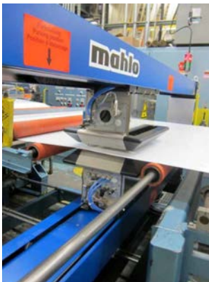
Fig. 2: Web gauging with Qualiscan QMS-12
