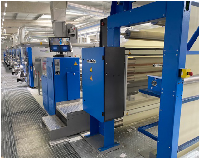
The Orthopac RVMC-15 is integrated into the new stenter frame.
