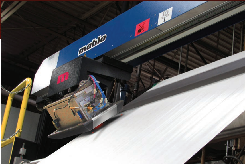
Mahlo custom engineered the scanner mount, adapting to available space on line #19.
