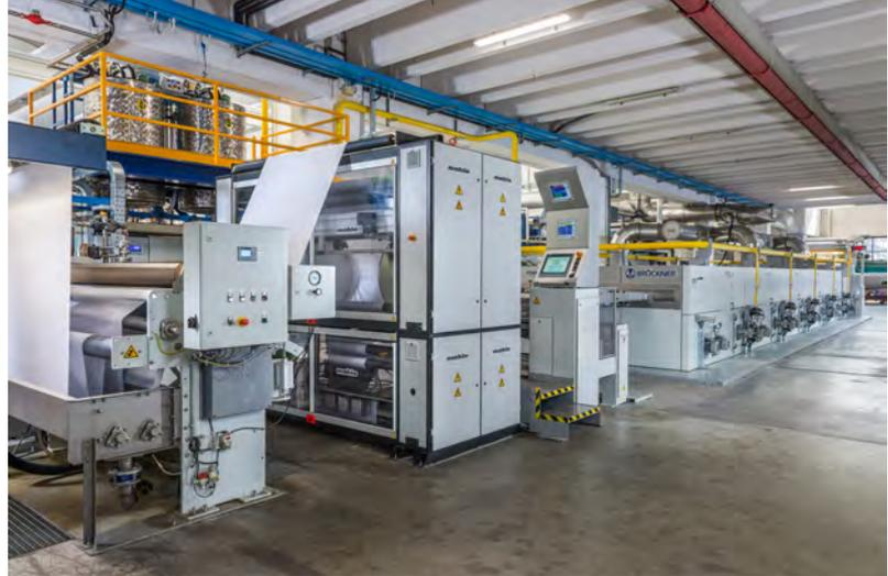
*Mahlo combination system with Orthomax RFMB and Optipac VMC process control on a stenter in the finishing area.*
