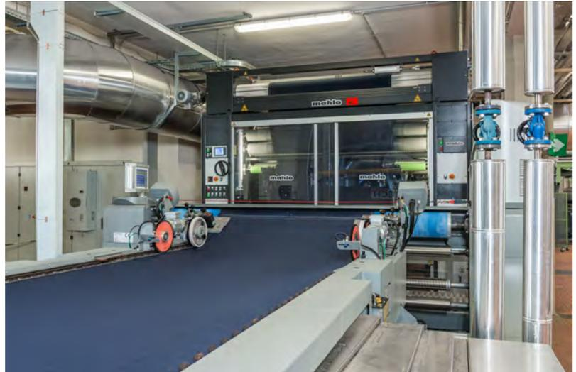
*The Orthomax removes web distortions before the stenter.*
