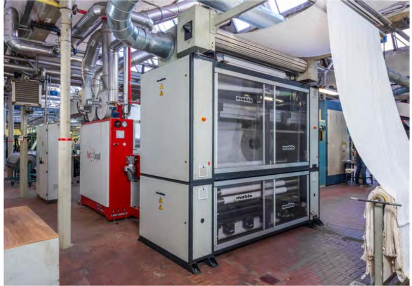
*The fusion of pin wheel and roller straightening device perfectly combines both technologies and provides amazing straightening results.*
