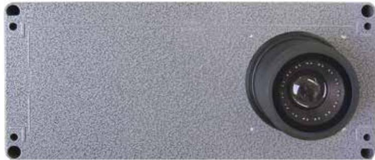
Traversing scanner with halogen lamp and spectrometer
