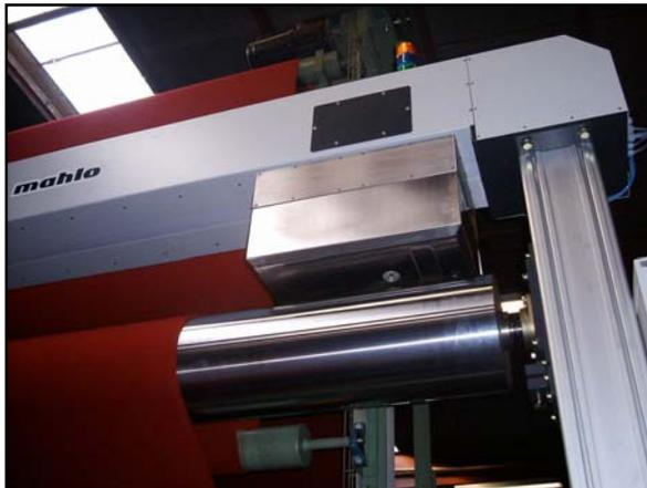
Installation picture of a MAHLO FMX sensor with Uniscan, working against a precision steel roll
