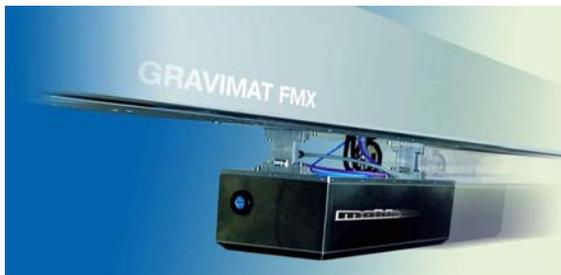
at 65 KV for minimum product composition sensitivity and best possible measurement accuracy in combination with small time constants, to allow for fast scanning across the web. For maintenance or transport of the unit, the x-ray tube can easily be powered off, avoiding any kind of exposure of machine or service personnel to unwanted radiation.
