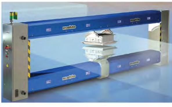
FIGURE 1. Typical on-line web-gauging system
